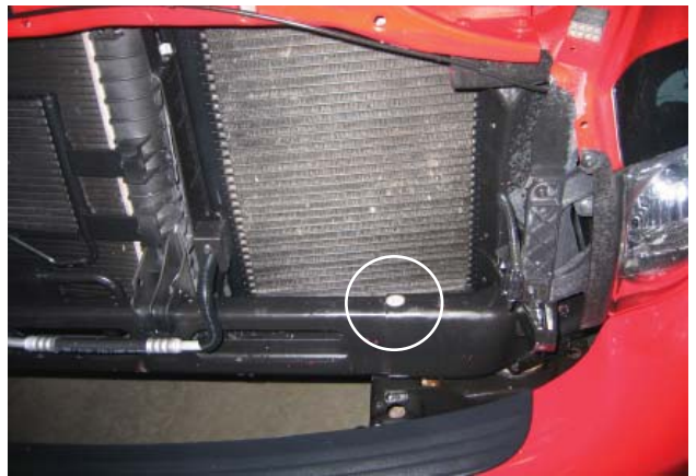
Removed Driver's Side Bolt
