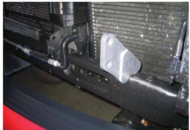
Installed Driver's Side I/C Bracket
