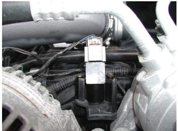
2-Bar MAP Sensor Installed
