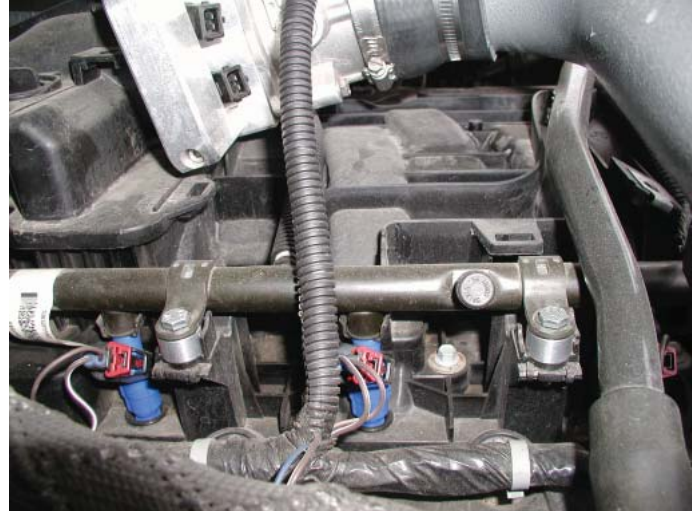
Fuel Rail Spacers Installed
