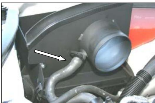
**7. Re-install the breather hose and speed clamp (#8) onto the nipple on the Quick Fit Panel. If you are working on a 6.1L, install the 1/2" x 90° elbow (#9) from the breather hose to the nipple on the Quick Fit Panel.**
