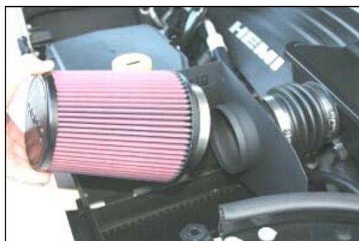
**8. Install the Airaid Premium Filter (#1) onto the tube on the Quick Fit Panels, and tighten the clamp.**
