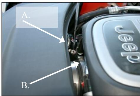
4. A.) Using the 10mm socket, remove the bolt that holds the stock intake system. B.) Loosen the hose clamp that holds the coupler to the throttle body.
