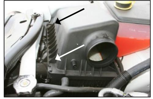
8. If you purchased an Airaid Jr. Kit, unhook the two clips and remove the factory air filter, and replace it with the Airaid Premium Filter supplied in the kit.
