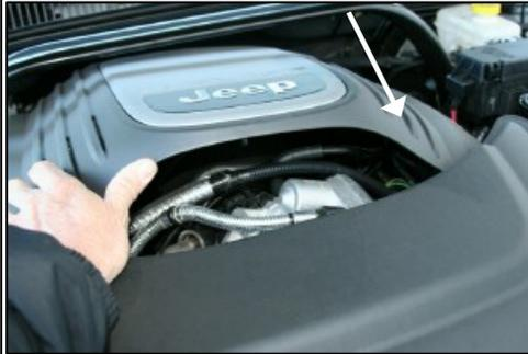
14. Re-install the engine cover by firmly pushing it back into the grommets.
