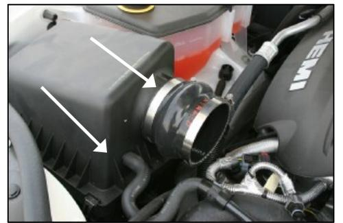
9. Reconnect the breather hose. Install the hump hose and two #60 hose clamps as shown. **Do not** tighten the clamps.
