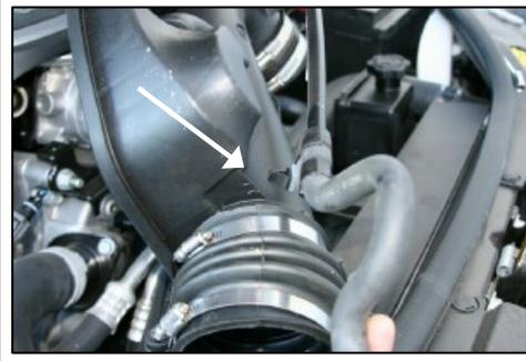
6. Slide the clip off of the intake tube that holds the breather line.
